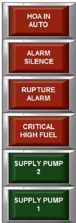
Correct the abnormal condition that is causing a flashing red LED graphic. The system will automatically restore the flashing LED graphic to its solid state.
