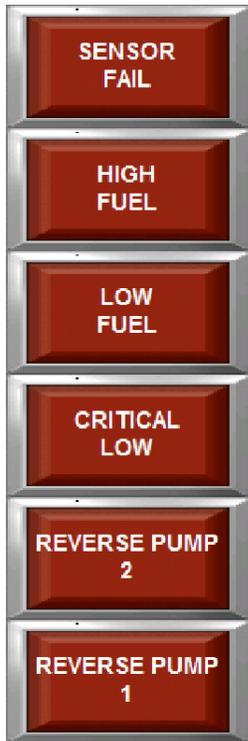
Correct the abnormal condition that is causing a flashing red LED graphic. The system will automatically restore the flashing LED graphic to its solid state.
